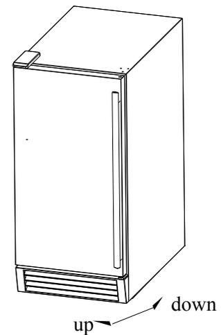
1. Place a carpenter's level on top of the unit to see if the ice maker is level from front to back and side to side .
